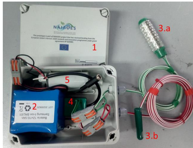
Figure 2 Urban Box prototype internal components
