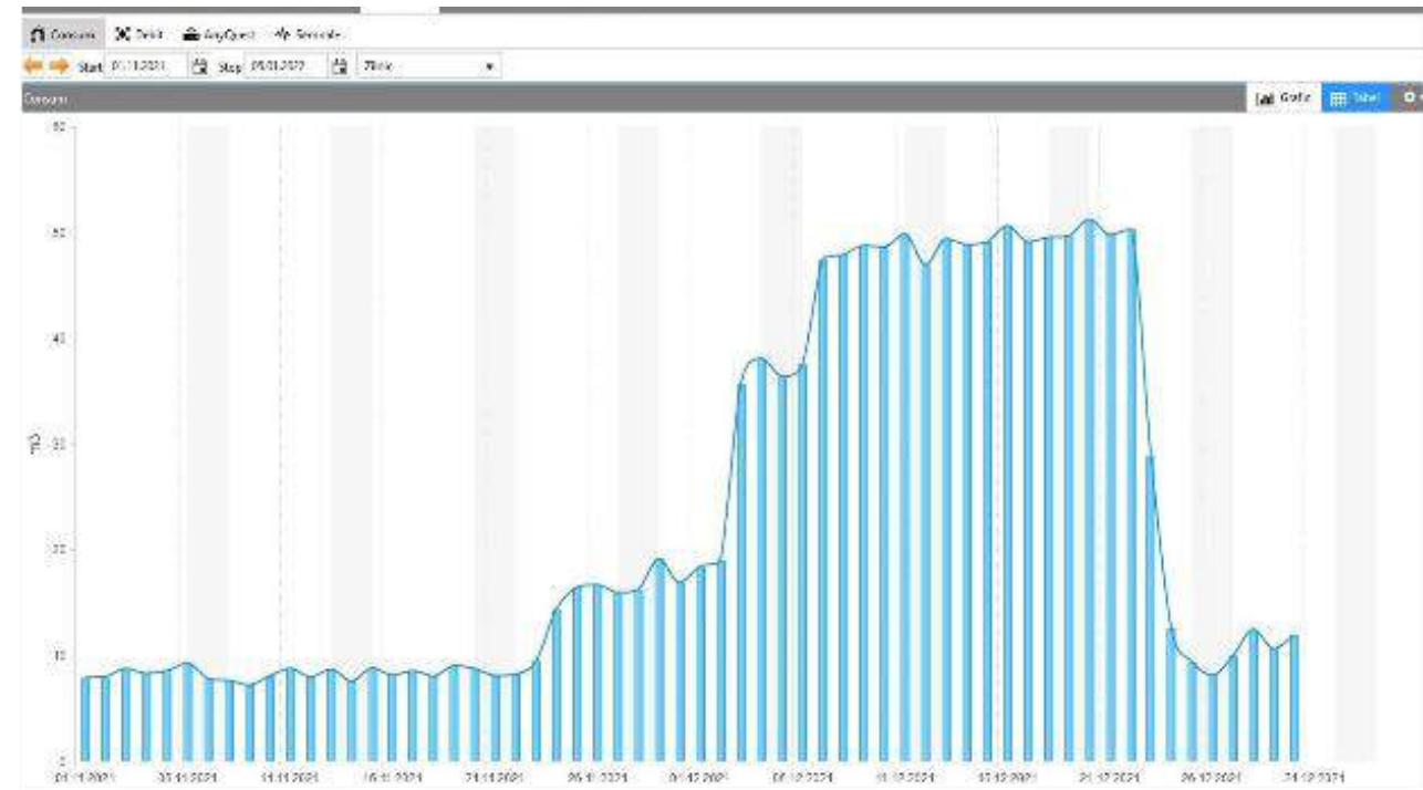
Large increase in flow at an end-user meter after a pipe burst in a high-rise building
