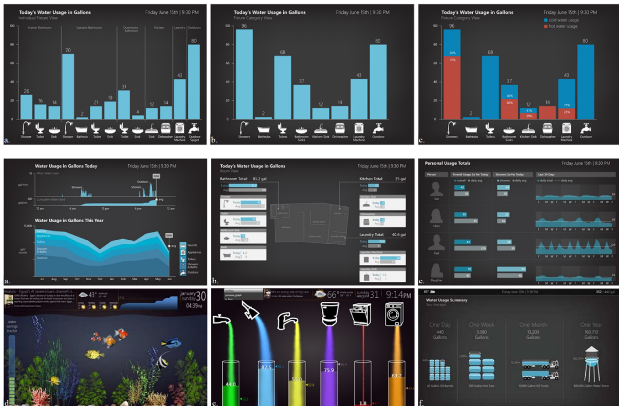
Figure 17: The water consumption displays designed by Froehlich et al., (2012). The designs provide views of consumption time granularity and comparisons, including self-monitoring, goal-comparison and social comparison. Moreover, consumptions are displayed by individual fixture; by fixture type; and by hot/cold water consumption breakdown. Additionally, they designed visually attractive presentations of water consumption including spatial presentation of water consumption (per room), consumption per household occupant, an abstract display that showed an aquarium that evolves in a positive manner when users water consume less water, a rainflow presentation of consumption, geographic comparisons that use maps to compare usage across an area and displays of metaphorical units based on the use of common, everyday objects such as a gallon jugs or oil trucks to depict usage.
